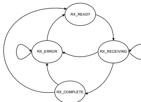
Figure 4: The Receiver State Diagram
