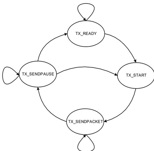
**Figure 5: The Transmitter State Diagram**
