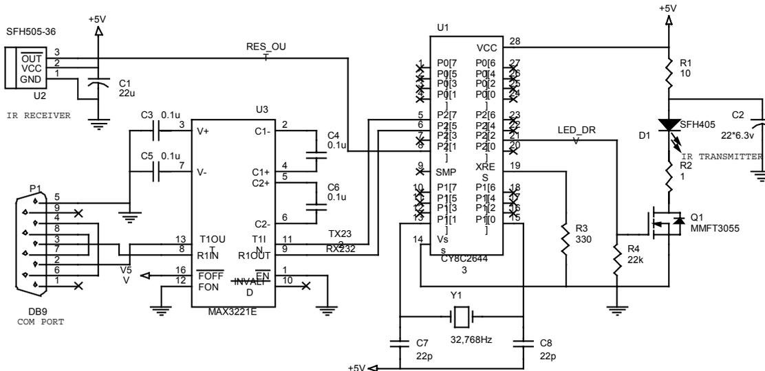
Figure 2: Codec Schematics
